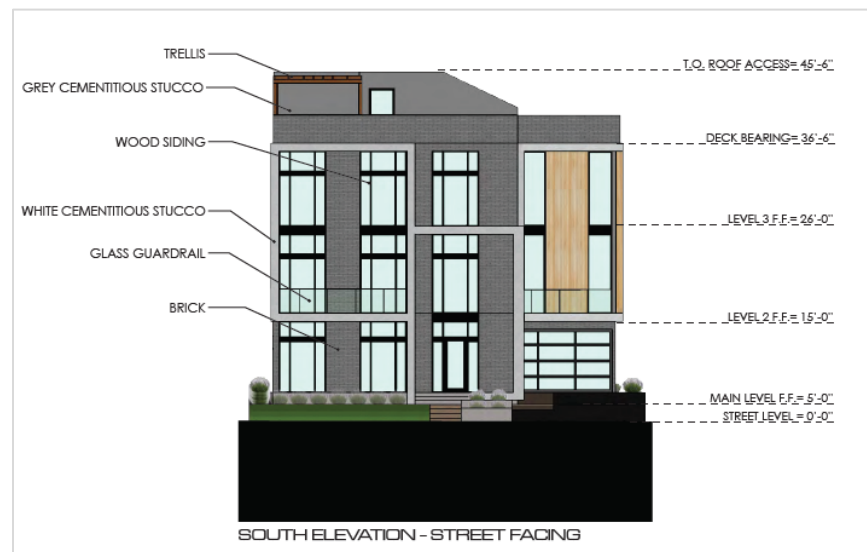
Figure 12 – Proposed front façade after revisions. Revised façade gained a prominent front entrance and established better connections with adjacent structures.
